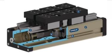
By pressure actuation of the opposing piston, the base jaws are guided by a carrier on the piston, and are set in motion. The synchronization of the jaw stroke is done with a rack and pinion principle.
