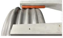
Pictured: Close-up of silicone rubber inserts on the gripper fingers.
