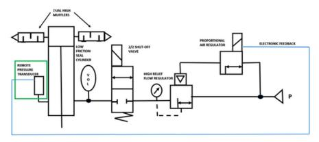
By measuring the pressure in the cylinder, we by pass any pressure drops through valving, regulators, ports and hoses. This provides the MOST accurate feedback to the Cordis and allows us to have accurate pressure control.
